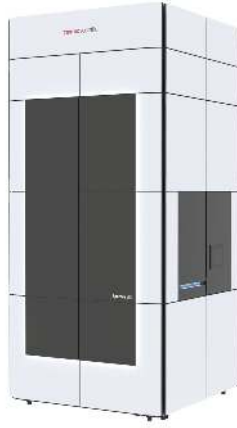
Figure 1.1. A Thermo Fisher Scientific Spectra scanning/transmission electron microscope, taken from Davies [1]. The column contains the electron gun, multiple electromagnetic lens systems, a phase plate, and a direct electron detector in a housing that exceeds two meters in height. Specimen loading, stage control, and image acquisition are automated, but alignment and calibration of the optical column still require expert intervention before each session.
